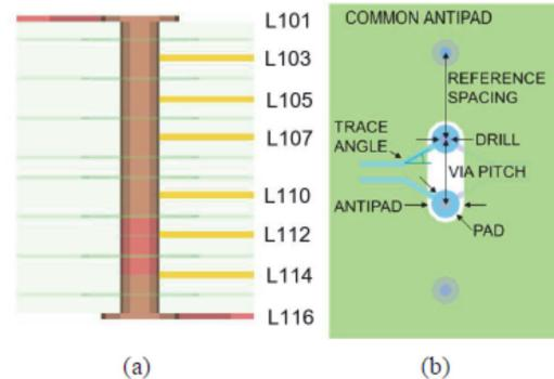
Figure 1. 16 Layer via PCB & Parameters
