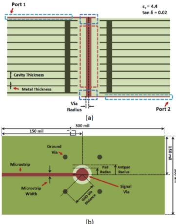
Fig. 1. Signal via in a 11 metal layer PCB with microstrip traces: (a) Side
