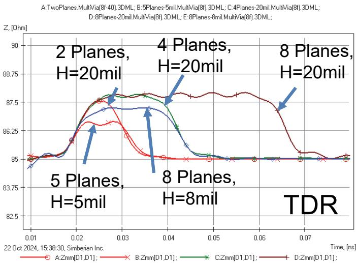
A:4Planes-20mil.MultVia[8f].3DML; B:TwoPlanes.MultVia[8f-40].3DML; C:8Planes-20mil.MultVia[8f].3DML; D:8Planes-8mil.MultVia[8f].3DML;
