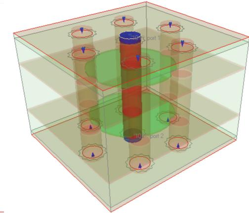
$$Dk = 3, D_{via}=8\text{mil}, D_{st}=40\text{mil}, s=21\text{mil} \rightarrow f_{cutoff} \approx 96.4 \text{ GHz} \quad (<\text{AWG30})$$
