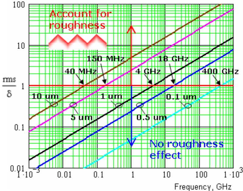
Fig. 5. Ratio of rms surface roughness values to skin depth in copper. Brown line – 10  $\mu\text{m}$ , magenta – 5  $\mu\text{m}$ , black 1  $\mu\text{m}$ , blue 0.5  $\mu\text{m}$ , cyan – 0.1  $\mu\text{m}$ . Roughness must be taken into account in model if the ratio is about 1 or greater. PCB and packaging interconnects may have rms roughness values between 10  $\mu\text{m}$  and 0.5  $\mu\text{m}$ .
