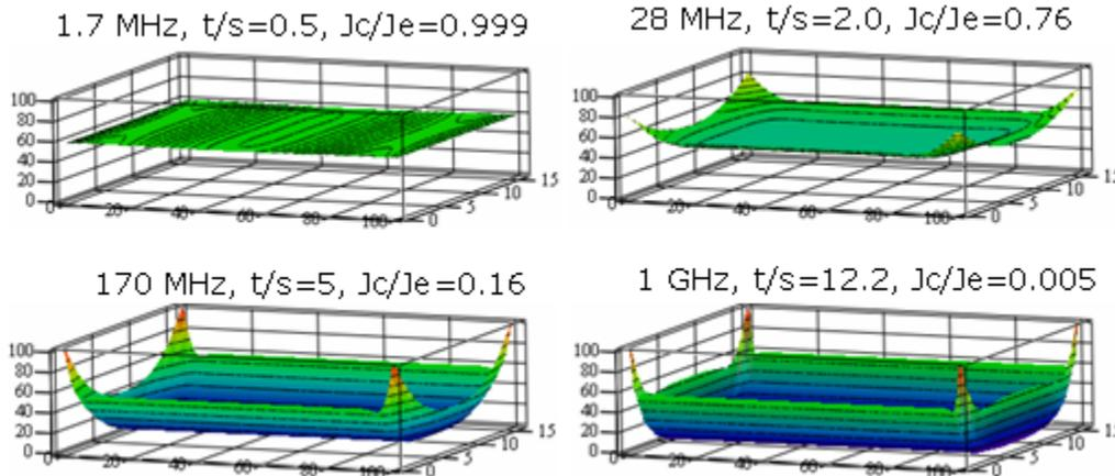
Fig. 3. Current density distribution over the cross-section of a 10 mil wide and 1 mil thick copper strip with voltage drop along the line 1  $\mu\text{V}/\text{m}$  for different frequencies.  $t/s$  is the strip thickness to the skin depth ratio,  $J_c/J_e$  is the ration of current density at the edge to the current in the middle. Computed with Trefftz finite elements [4]
