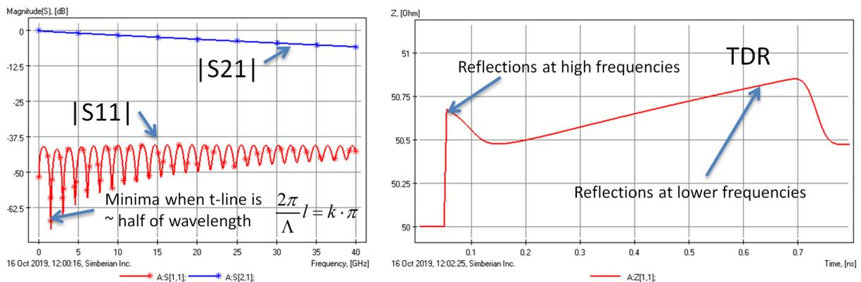
Both ends of the transmission line segment are terminated by 50 Ohm (exactly). Magnitudes of the reflection |S11| and transmission |S21| parameters are shown on the left plot and corresponding TDR on the right plot (reflection from 20 ps step response in Ohm). S-parameters are shown in dB
