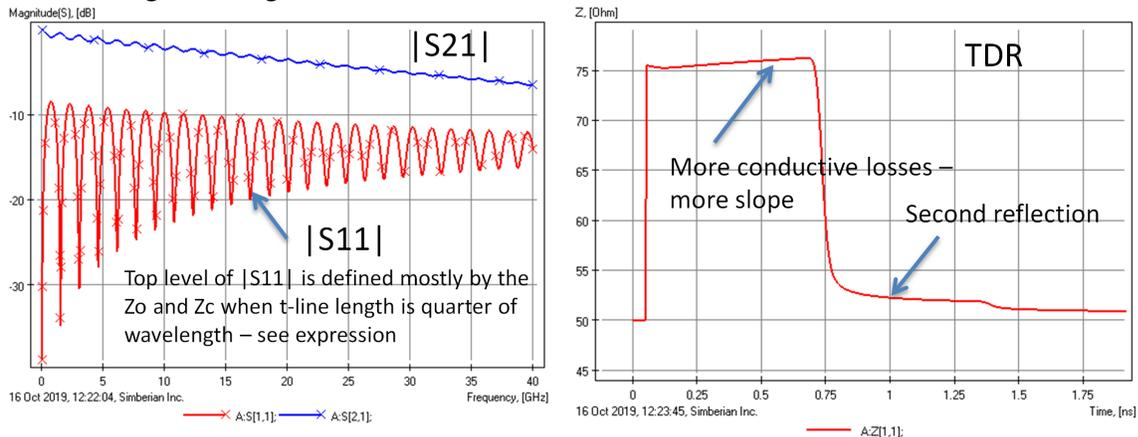
On S-parameter plot it looks very similar to the previous case. Though, it has more conductive losses and the TDR goes up, instead of down, and shows more resistance (slope up) in the narrow transmission line as expected. In both “reflective” cases only one or two reflections are significant – it disappears quickly due to the absorption losses (losses are our friend in such reflective cases).
