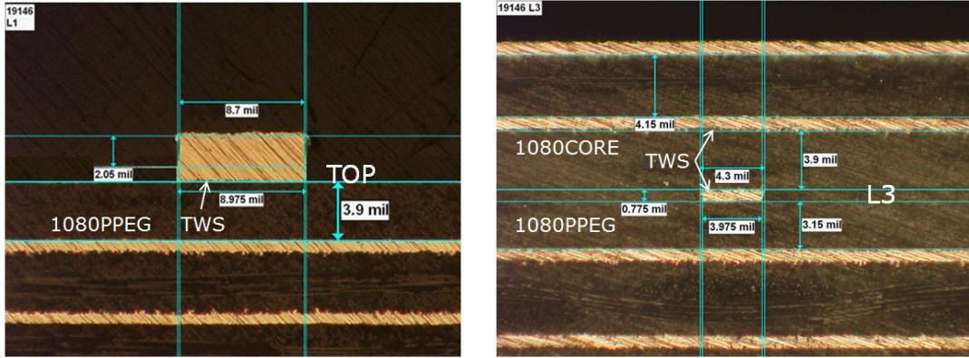
*Fig. 3. Micro-photographs of cross-sections and dimensions for top microstrip (left) and strip line in layer L3 (right).*
