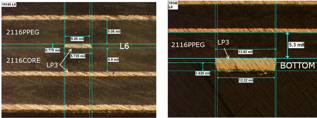
*Fig. 4. Micro-photographs of cross-sections and dimensions for bottom microstrip (right) and strip line in layer L6 (left).*
