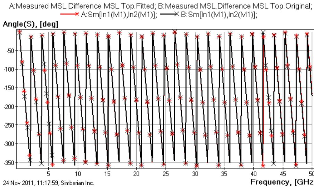
Fig. 9. Generalized modal transmission phase for 4-inch segment of microstrip line in top layer (RTF, 1080). Original data – red stars, fitted results – black crosses.
