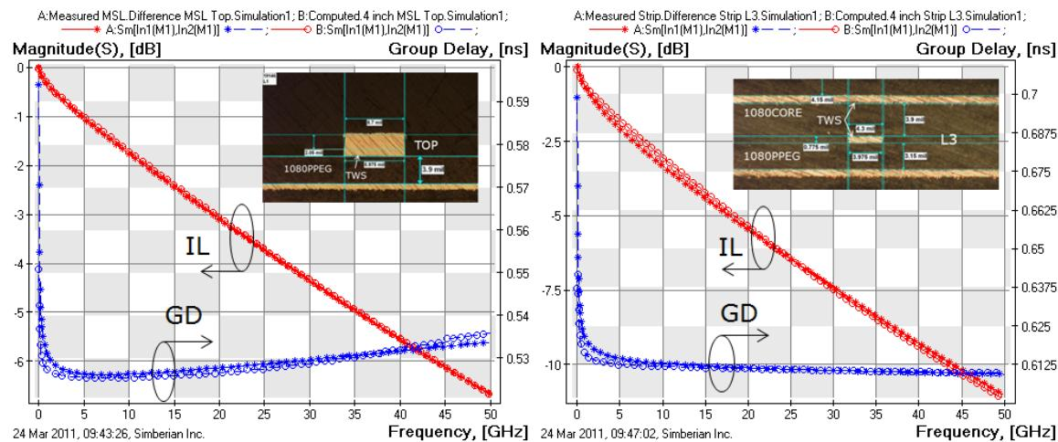
*Fig. 21. Measured (stars) and modelled (circles, MHCC roughness model) insertion loss (IL, red curves) and group delay (GD, blue curves) of 4 inch microstrip line in top layer (left) and strip line in layer L3. Foil RTF, laminate 1080, adjusted Dk,  $\Delta = 0.35$  and RF=2.6.*
