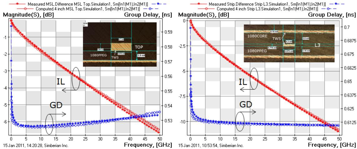
*Fig. 20. Measured (stars) and modelled (circles, Simbeor roughness model) insertion loss (IL, red curves) and group delay (GD, blue curves) of 4 inch microstrip line in top layer (left) and strip line in layer L3 (right). Foil RTF, laminate 1080, adjusted Dk,  $\Delta = 0.35$  and RF=2.8.*
