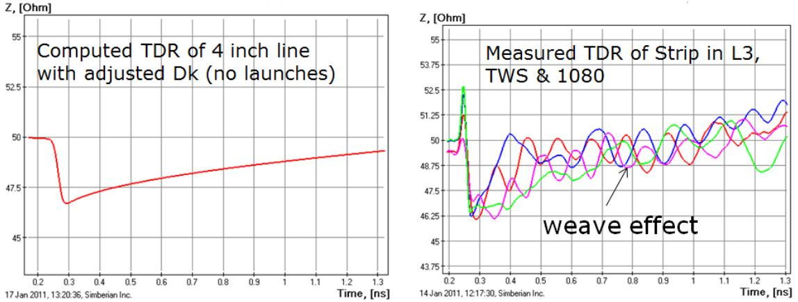
*Fig. 13. Computed TDR plot for a 4-inch strip line in layer L3 with adjusted Dk (left plot) and measured TDR (computed from measured S-parameters) for all strip line structures in layer L3.*
