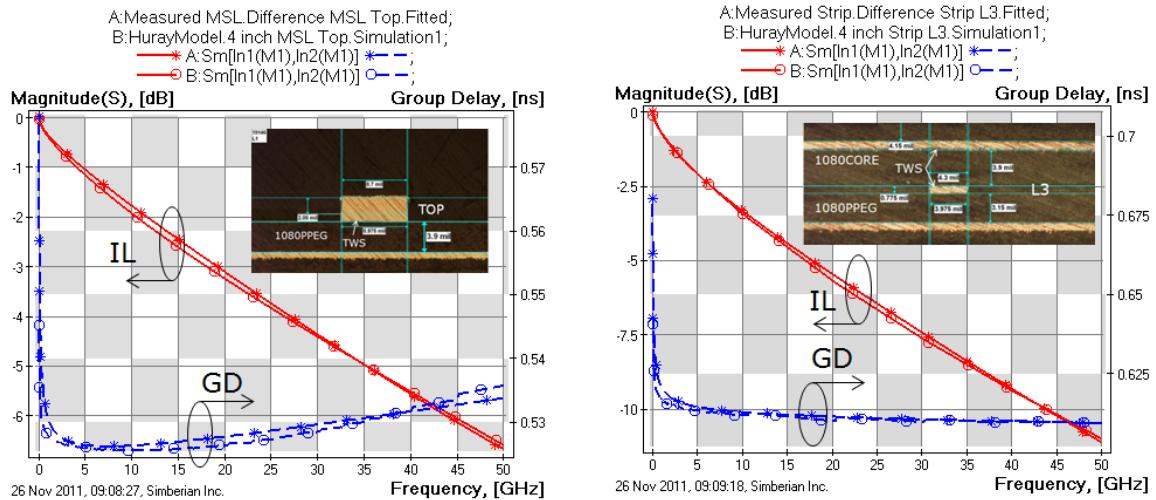
Fig. 22. Measured (stars) and modelled (circles, Huray's snowball roughness model) insertion loss (IL, red curves) and group delay (GD, blue curves) of 4 inch microstrip line in top layer (left) and strip line in layer L3. Foil RTF, laminate 1080, adjusted  $D_k$ , ball radius 0.5  $\mu\text{m}$ , tile size 4.98  $\mu\text{m}$ ,  $N_b=15$ .
