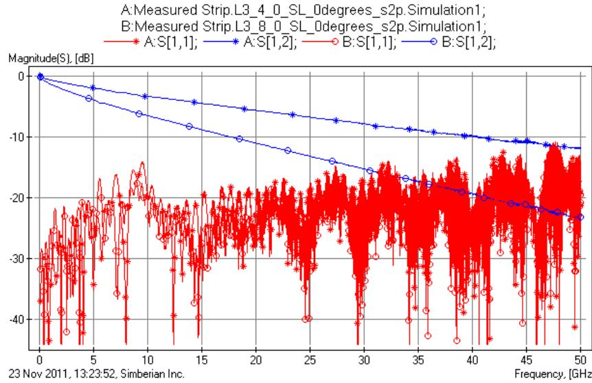
*Fig. 6. Insertion loss (blue) and reflection loss (red) for 4-inch (stars) and 8-inch (circles) segments of strip line in layer L3 (RTF, 1080). Data quality is acceptable ( $QM > 90\%$ ). Data provided by INAOE.*
