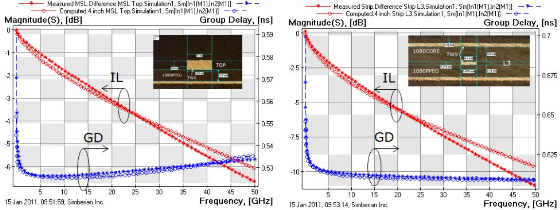
Fig. 18. Measured (stars) and computed (circles) generalized modal insertion loss (IL) and group delay (GD) of 4 inch microstrip line in top layer (left plot) and strip line in layer L3 (right plot). Foil RTF, laminate 1080, Dk of laminates are adjusted, roughness model parameters are measured with profilometer ( $Rq=2.6\text{ }\mu\text{m}$ ,  $RF=1.85$ ).
