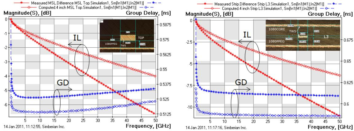
*Fig. 10. Measured (stars) and preliminary computed (circles) generalized modal insertion loss (IL, red curves) and group delay (GD, blue curves) of 4 inch microstrip line in top layer (left plot) and strip line in layer L3 (right plot). Foil RTF, laminate 1080.*
