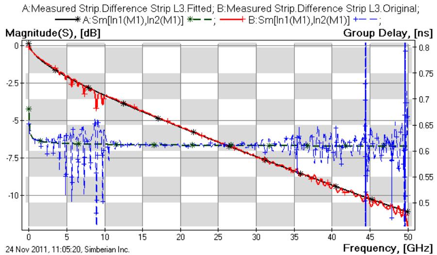
Fig. 8. Generalized modal insertion loss (red and black lines, left axis) and group delay (blue and green lines, right axis) for 4-inch segment of strip line in layer L3 (RTF, 1080). Original data – red and blue lines, fitted results – black and green lines.
