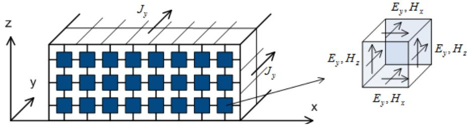
Fig. 14. Trefftz finite element model of the three-layer conductor (elements have different size along the Z-axis).
