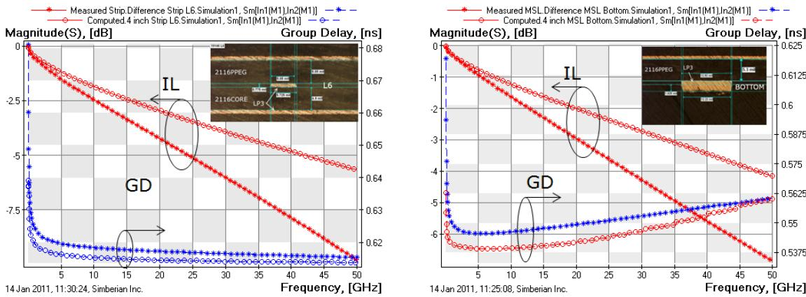
*Fig. 11. Measured (stars) and preliminary computed (circles) generalized modal insertion loss (IL, red curves) and group delay (GD, blue curves) of 4 inch strip line in layer L6 (left plot) and microstrip line in bottom layer (right plot). Foil VLP, laminate 2116.*
