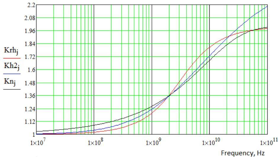
*Fig. 15. Comparison of roughness correction coefficients. MHCC model - red line,  $\Delta = 1\text{um}$   $RF=2.0$ . Huray's snowball model – blue line, sphere radius  $0.85\text{um}$ , tile size  $11\text{ um}$ ,  $N_s=20$ . Simbeor model – black line,  $\Delta = 1\text{um}$   $RF=2.0$ .*
