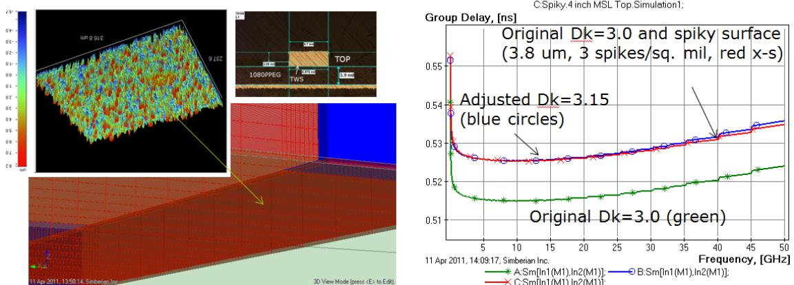
Fig. 17. Possible way to simulate capacitive effect of roughness – add spikes to rough surface of microstrip line. Size and number of spikes are adjusted to match measured group delay.
