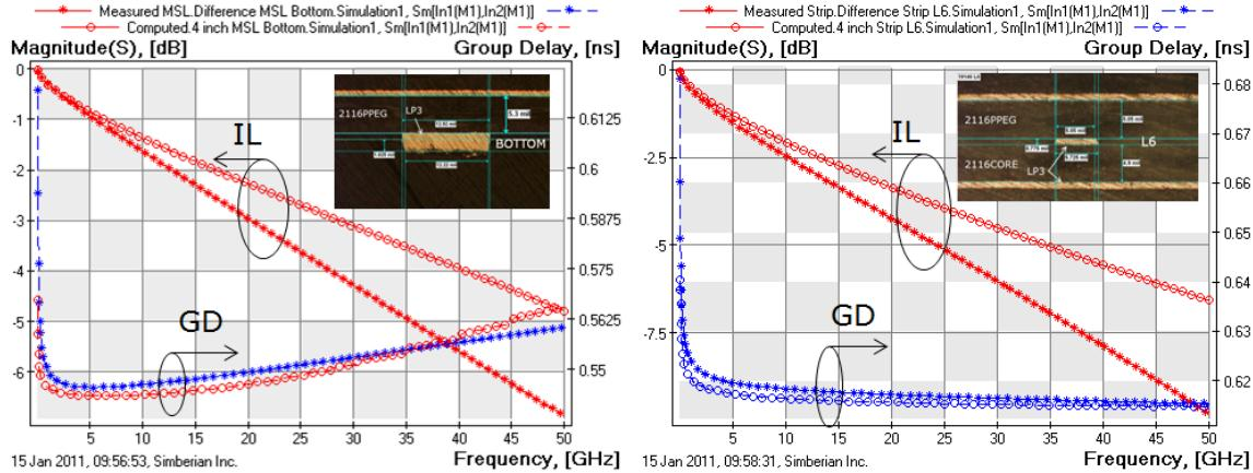
Fig. 19. Measured (stars) and computed (circles) generalized modal insertion loss (IL) and group delay (GD) of 4 inch microstrip line in bottom layer (left plot) and strip line in layer L6 (right plot). Foil VLP, laminate 2116, Dk of laminates are adjusted, roughness model parameters are measured with profilometer ( $Rq=0.68\text{ }\mu\text{m}$ ,  $RF=1.3$ ).
