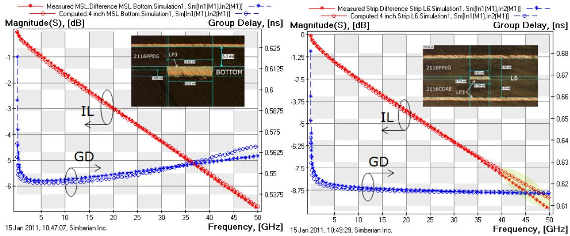
*Fig. 23. Measured (stars) and modelled (circles, Simbeor roughness model) insertion loss (IL, red curves) and group delay (GD, blue curves) of 4 inch microstrip line in top layer (left) and strip line in layer L3 (right). Foil VLP, laminate 2116, adjusted  $Dk$ ,  $\Delta = 0.11$  and  $RF=7$ .*
