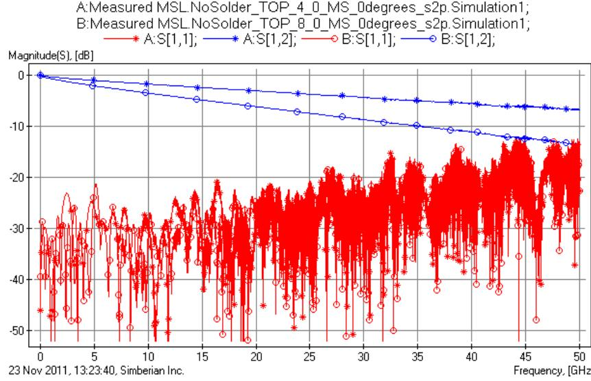
*Fig. 5. Insertion loss (blue) and reflection loss (red) for 4-inch (stars) and 8-inch (circles) segments of microstrip line in the top layer (L1, RTF, 1080). Data quality is acceptable ( $QM > 90\%$ ). Data provided by INAOE.*
