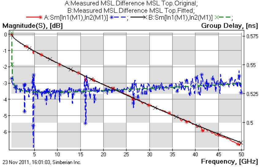
Fig. 7. Generalized modal insertion loss (red and black lines, left axis) and group delay (blue and green lines, right axis) for 4-inch segment of microstrip line in top layer (RTF, 1080). Original data – red and blue line, fitted results – black and green lines.
