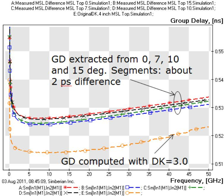
*Fig. 12. Generalized modal group delay (GD) of 4 inch microstrip line in top layer extracted for 0, 7, 10 and 15 deg. traces (computed from fitted phase). GD computed with  $Dk=3.0$  is shown by yellow line (circles) and consistently lower.*
