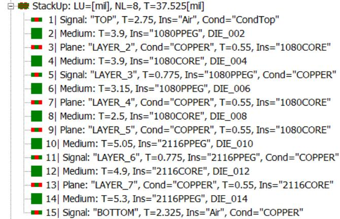
*Fig. 2. Test board stackup.*
