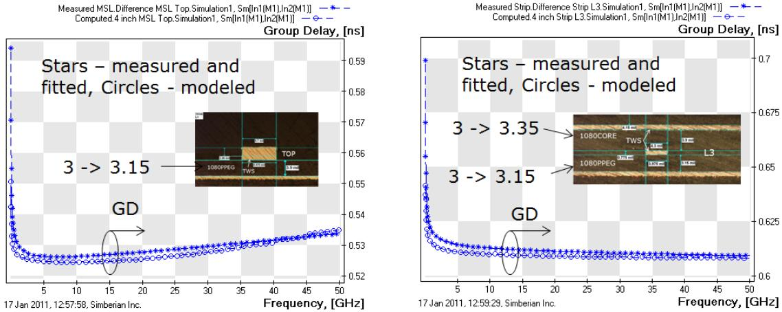
Fig. 16. Measured (stars) and computed with adjusted  $Dk$  (circles) generalized modal group delays (GD) of 4 inch microstrip line in top layer (left plot) and strip line in layer L3 (right plot). Foil RTF, laminate 1080.
